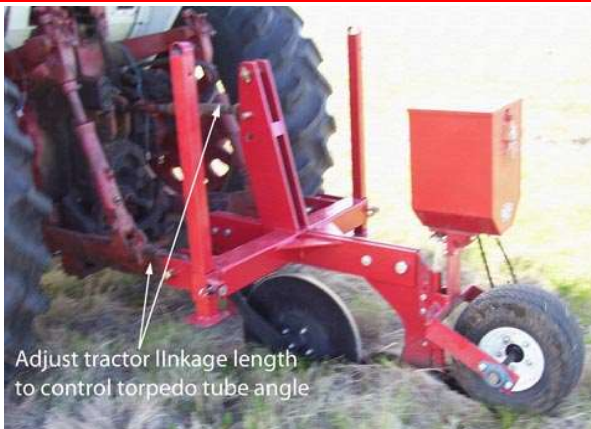
Figure 11: Adjustment of tractor link to control torpedo tube angle
